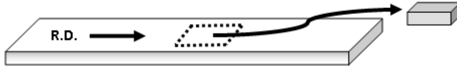
Fig. 3.4. A schematic drawing showing a rolled sample and specimen gathered for metallography
