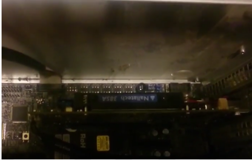
Figure 14: FPGA connected to host main board PCI-express slot
