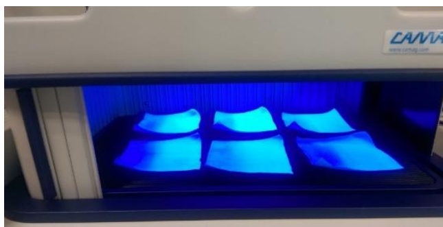
Figure 2.5. UV bleaching test set-up performed on textile in UV cabin.
