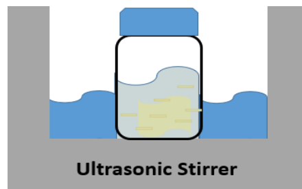
Figure 1.5. Chemical bath deposition process by ultrasonic stirrer.
