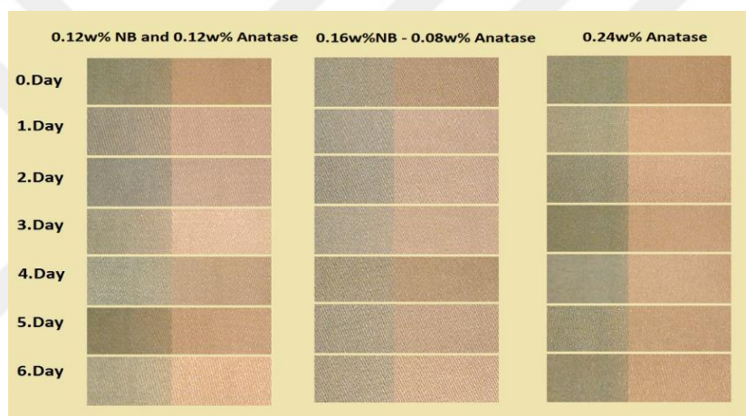
Figure 3.28. The stain bleaching tests conducted on finishing solution as compared to 0.24wt% nano-boron, 0.08wt% anatase doped with 0.16wt% nano-boron and 0.12wt% anatase doped with 0.12wt% nano-boron.
