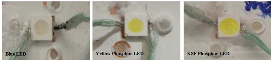
Figure 64 - Thermocouple arrangements of attaches the LEDs.
