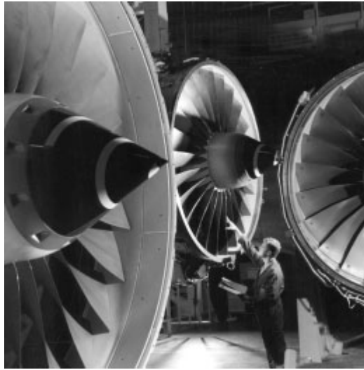
Figure 1.6: Front fans of commercial Rolls-Royce engines made of Ti-6Al-4V (Rolls Royce plc., Derby, UK)
