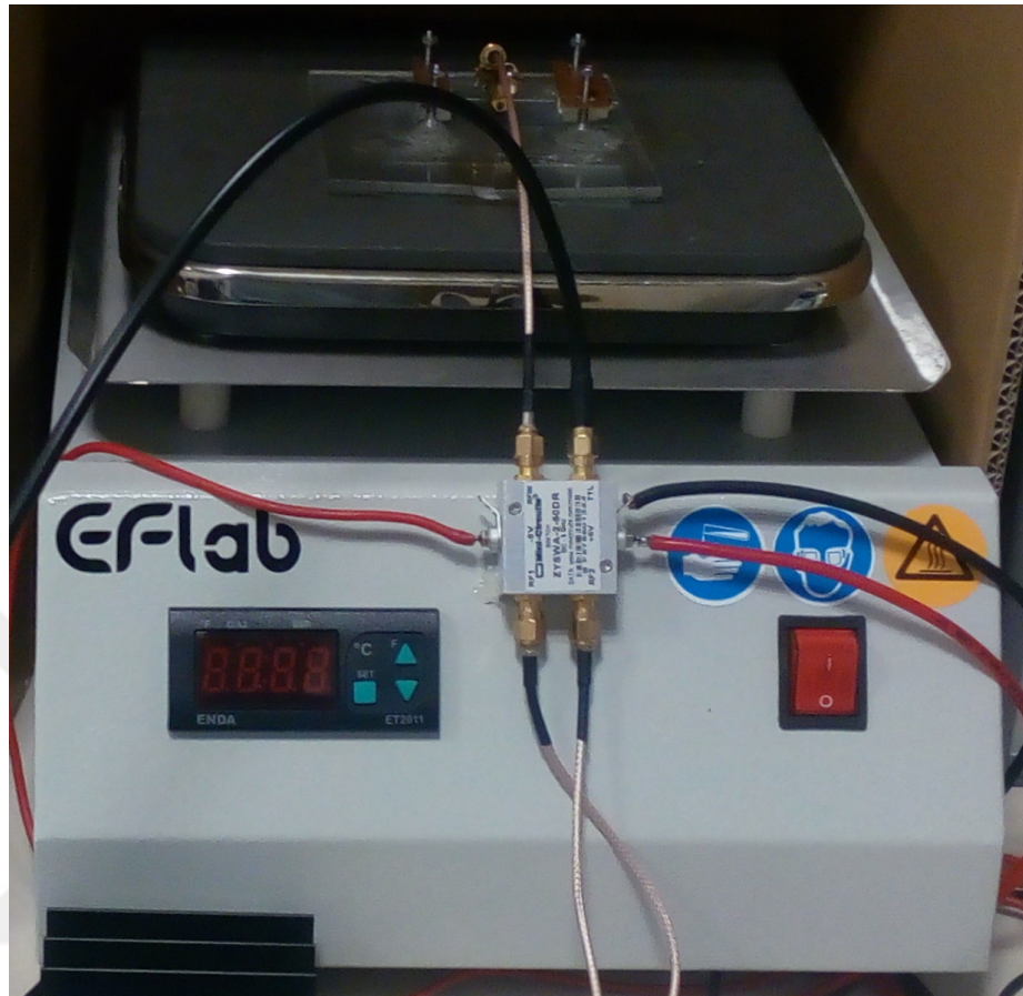
Figure 16: The commercial temperature control system for keeping the temperature at 37\pm 0.5^\circ\text{C} .
