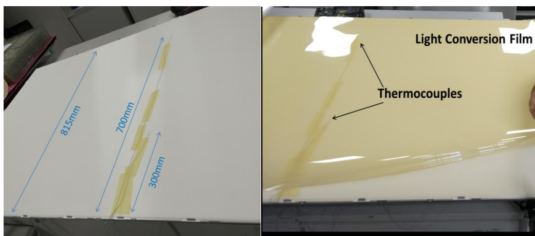
Figure 59: Thermocouples Connections between Colour Conversion Layer and DP
