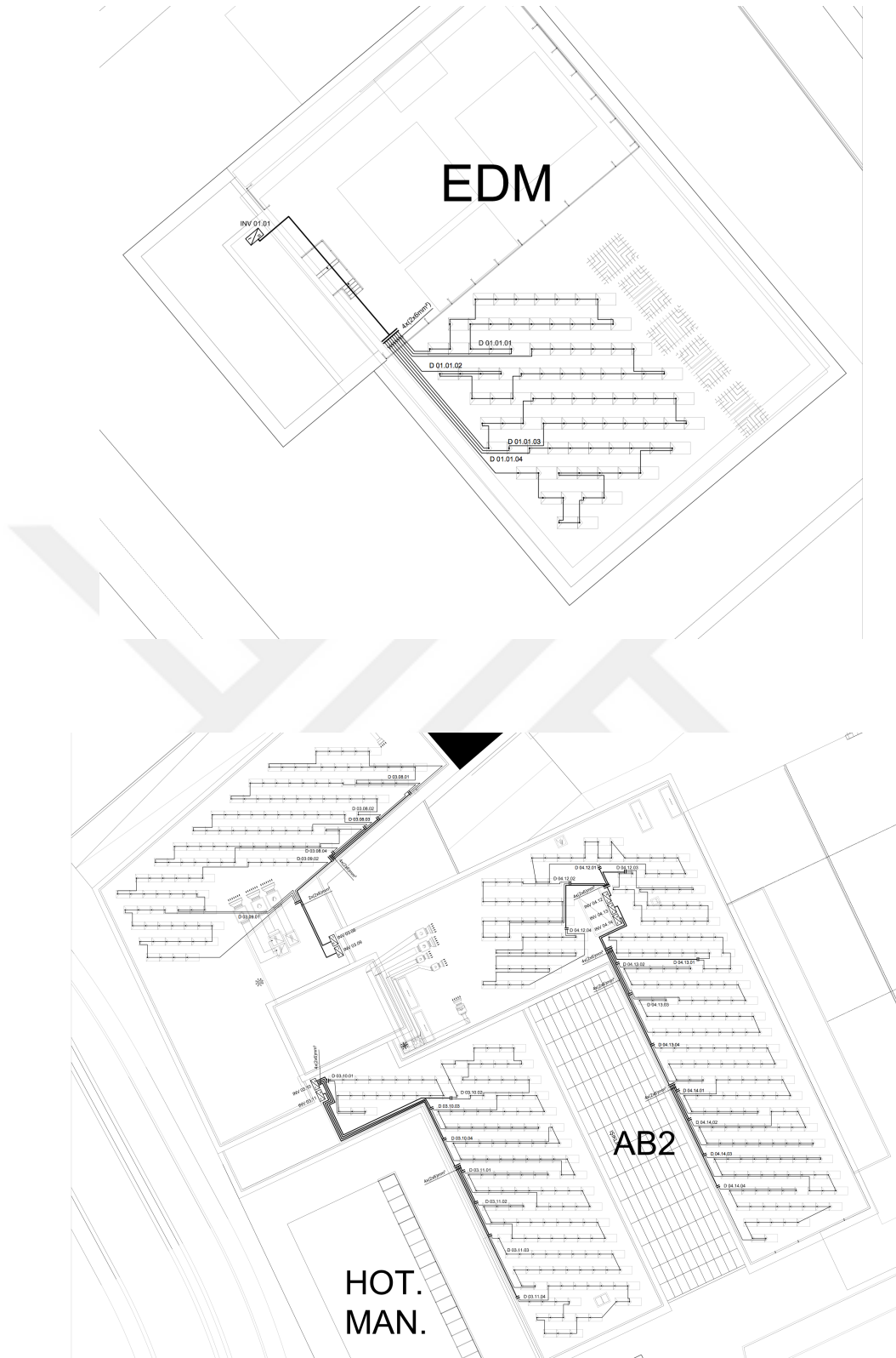
Figure 3-12 String Connections, PV Module Placement, AC and DC Cabling Routes of EDM and Engineering Building
