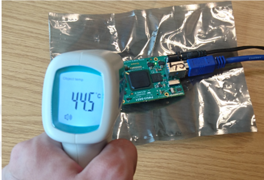
Figure 29: Temperature Measurement of FPGA.
