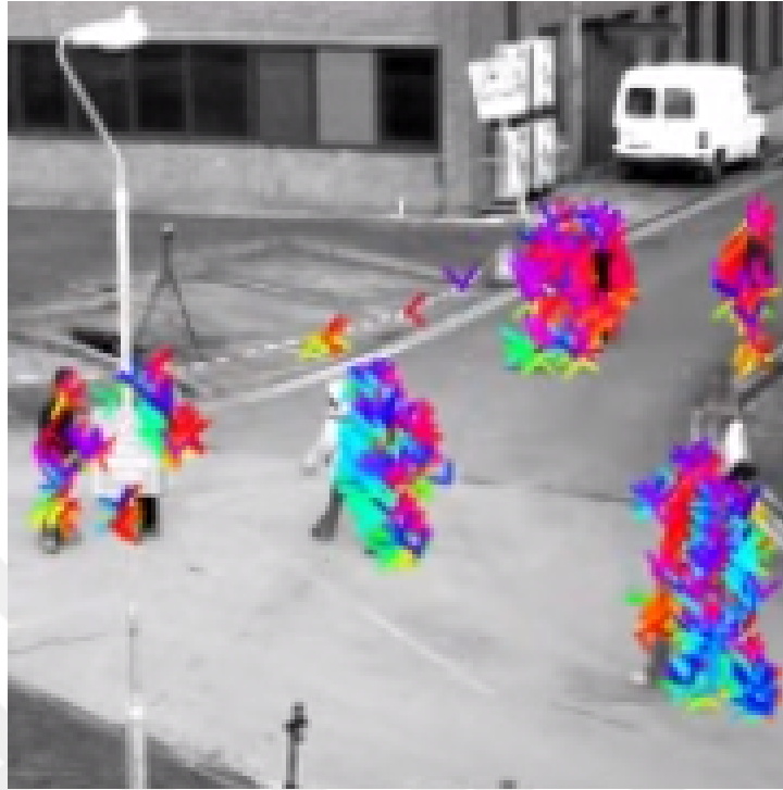
Figure 17: Output of the Optical Flow Algorithm.
