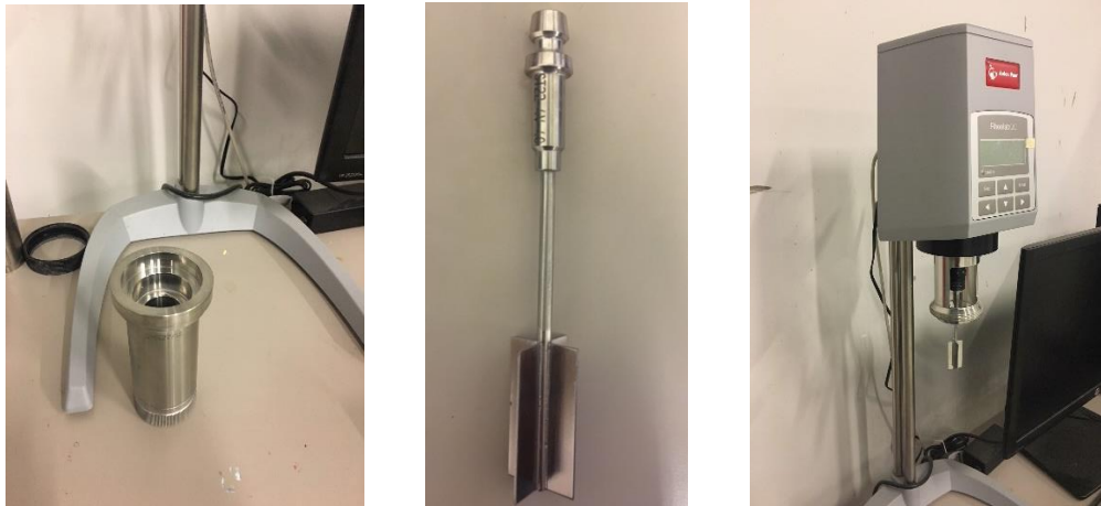
Figure 3-1 Image of the outer cylinder, the coaxial vane, and the rheometer device
