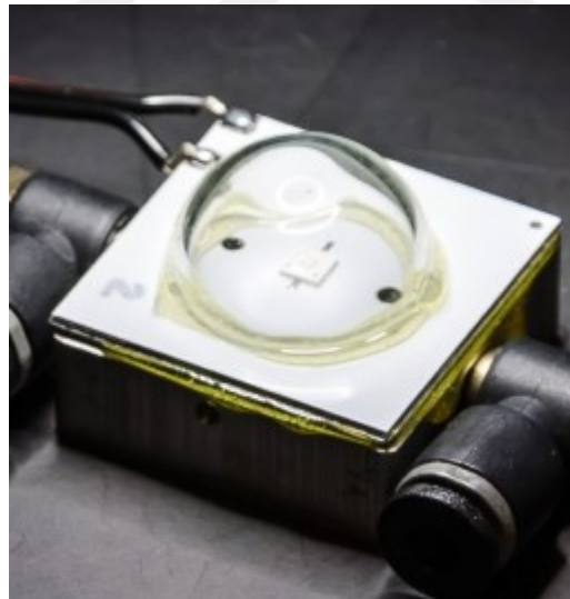
Figure 3-5: Blue LED chip with a glass dome
