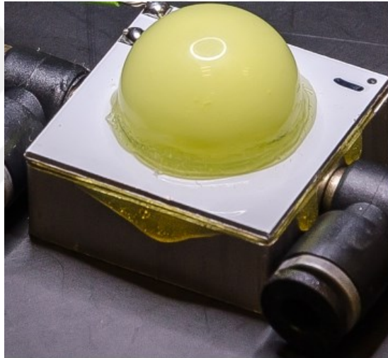
Figure 3-8: Remote phosphor coated LED package
