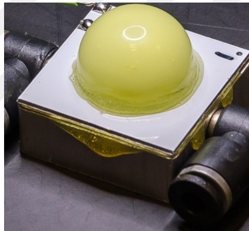
Figure 3-16: Remote phosphor coated liquid injected LED package
