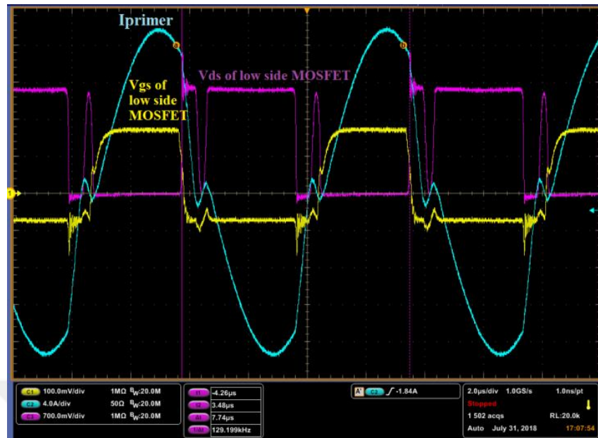
Figure 3.11: S2 drain-source voltage, gate input voltage and primer current with conventional method @ P_{out} = 1600 W, V_{out} = 160 V, f_{sw} = 130 kHz, \alpha = 1 \mu s
