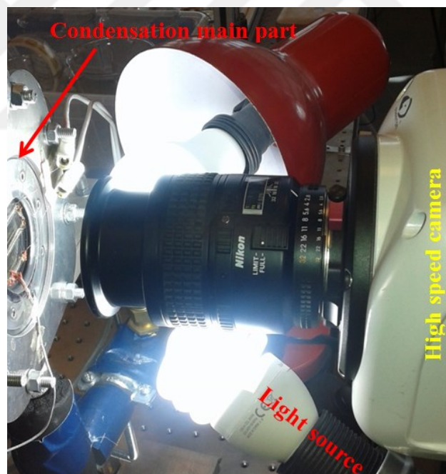
Figure B-2: High-speed camera with lamps lights during the condensation test
