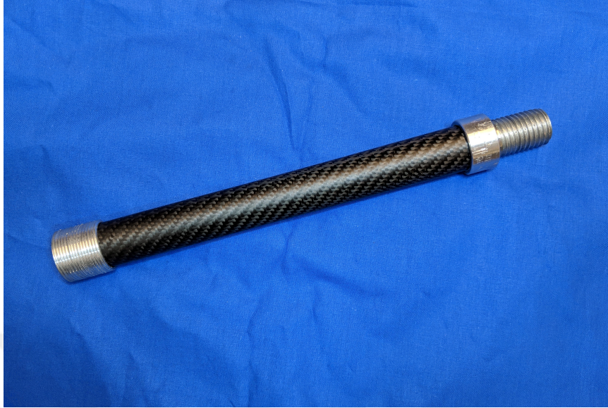
Figure 37: Additional expendable members designed to connect carbon-fibre members with aluminium members as placed on carbon-fibre tube
