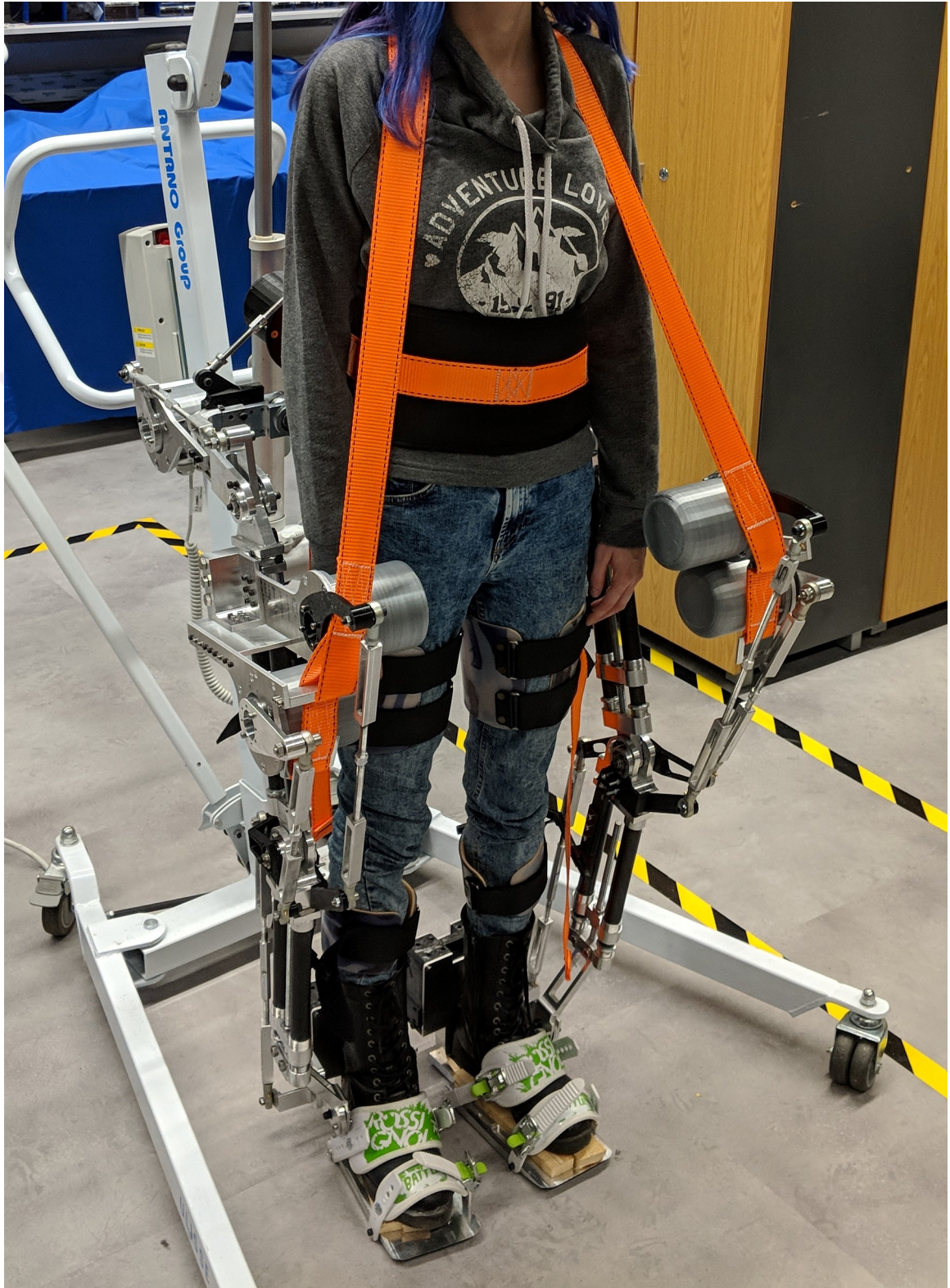
Figure 44: Manufactured version 1.0 with mock actuators, on a healthy female subject
