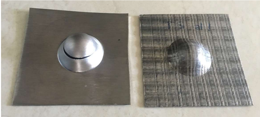
Figure 3.2.6: Samples formed after erichsen tests
