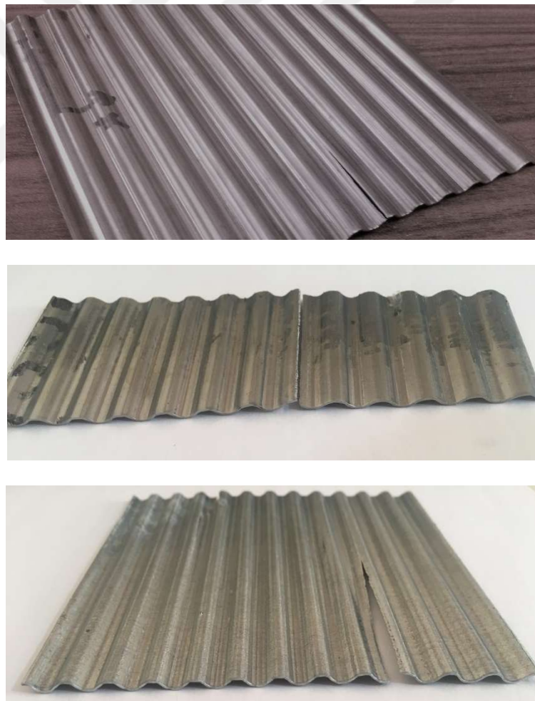
Figure 2.3: Fractures observed in (a) AISI 304, (b) Ti-15V-3Cr-3Sn-3Al and (c) commercially pure zinc
