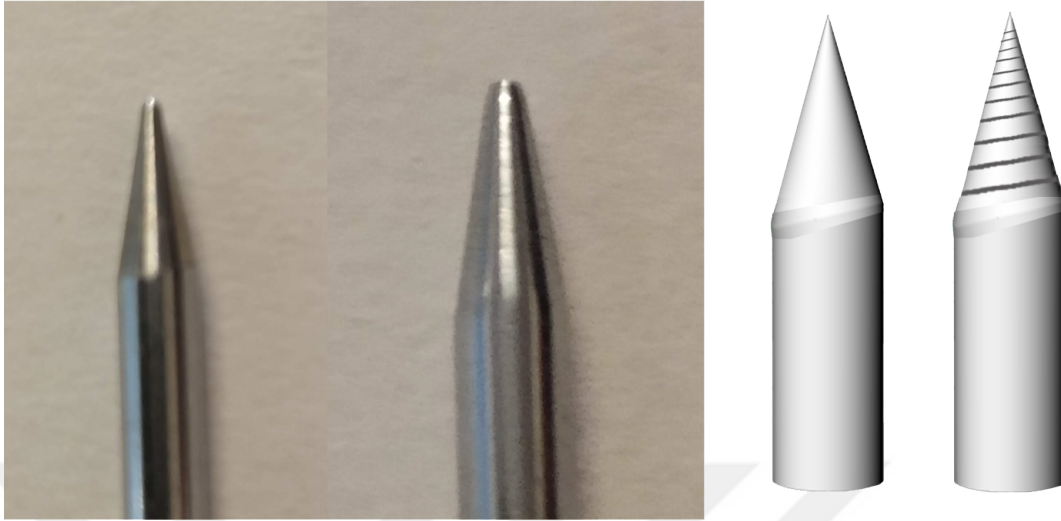
Figure 34: The trapezoid in the bottom base and winding-like lines on the worked area of the needle
