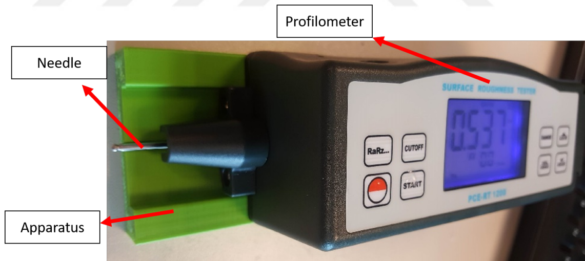
Figure 30: R_z and R_a measurement experiment setup: The needle is inserted into the cavity of the apparatus. Thus, the profilometer detects and measures the side surface of the needle as a flat surface.
