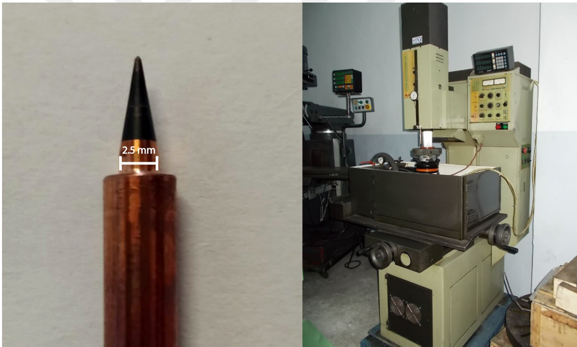
Figure 32: Copper electrode mold and plunge erosion machine (AJAN983)
