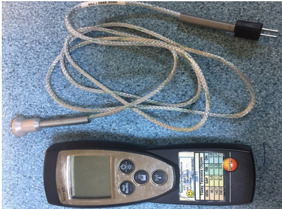
Figure 3.4: Portable surface temperature measurement instrument.
