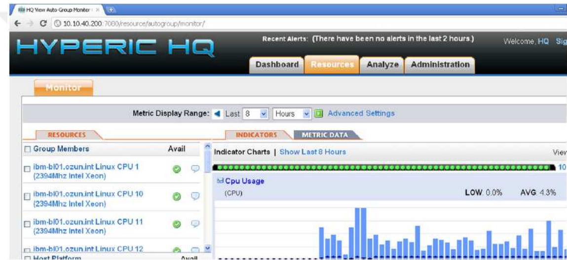
Figure 15: Overall (or per process) CPU, memory network and other resource usages can be tracked with Hyperic for cloud service accounting.
