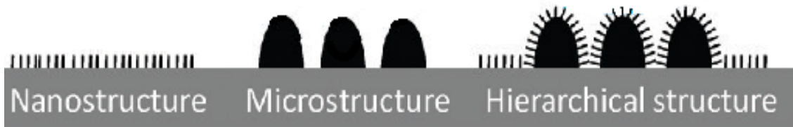
Figure 6-7 The surface roughness structures.
