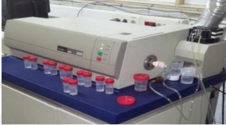
Figure 5-2 Mass spectrometry equipment with ICP ionization source.
