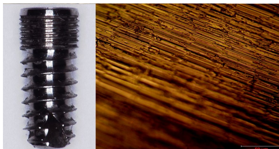
Figure 6-2 Microscopic images for baseline machined dental implant.
