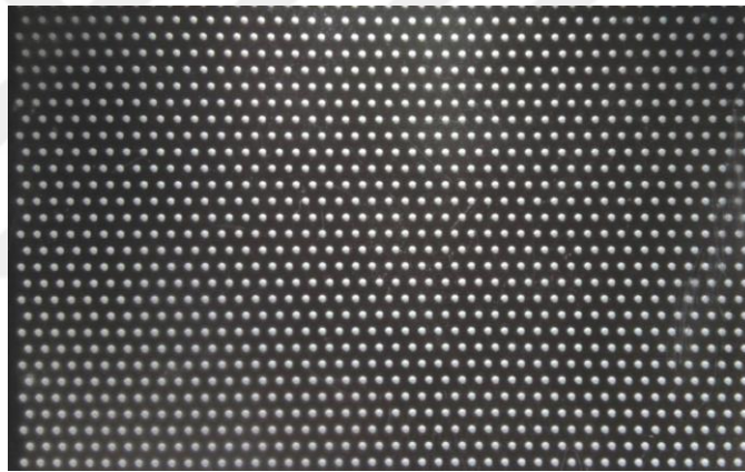
Figure 11: Top view of dot-patterned LGP.
