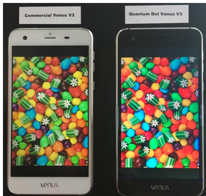
Figure 45: Color quality difference of the produced displays. (left) Commercial product contains standard white LED in BLU, (right) QD film embedded product.
