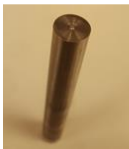
Figure 3.2 The flat tip welding tool used in this study
