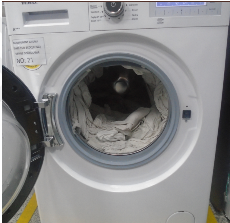
Figure 3: Washing Machine with unbalanced load
