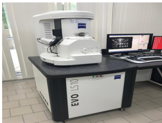
Figure 3.6: Scanning electron microscope (SEM), used for microstructural characterizations.
