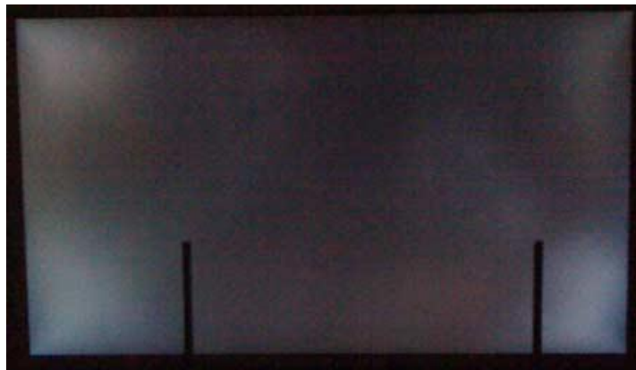
Figure 9: Thermal mura (corner mura) of 42” LED module [9]
