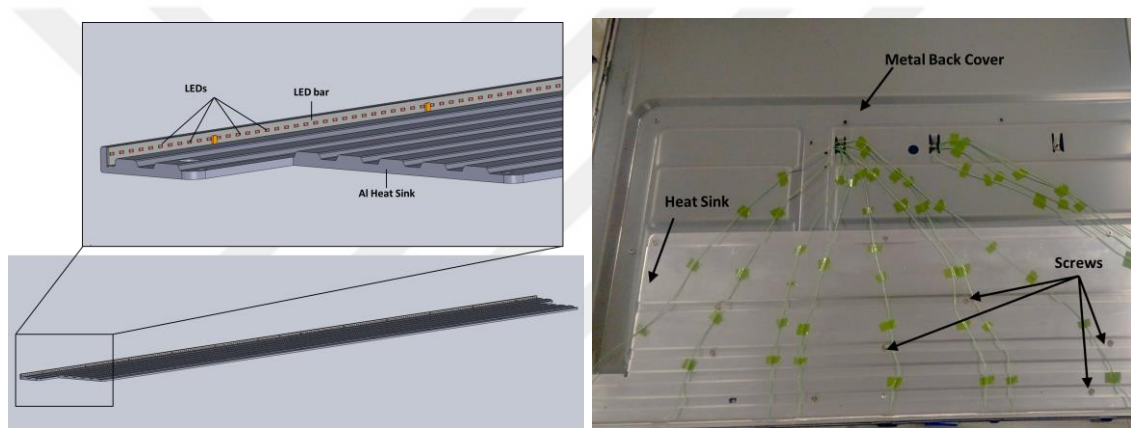
Figure 21: Aluminum heat sink with a LED bar [6]
