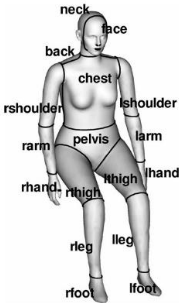
Figure 1.2. Scanned manikin body divided into sixteen segments. Face and neck constitute the head segment (Sørensen and Voigt, 2003)
