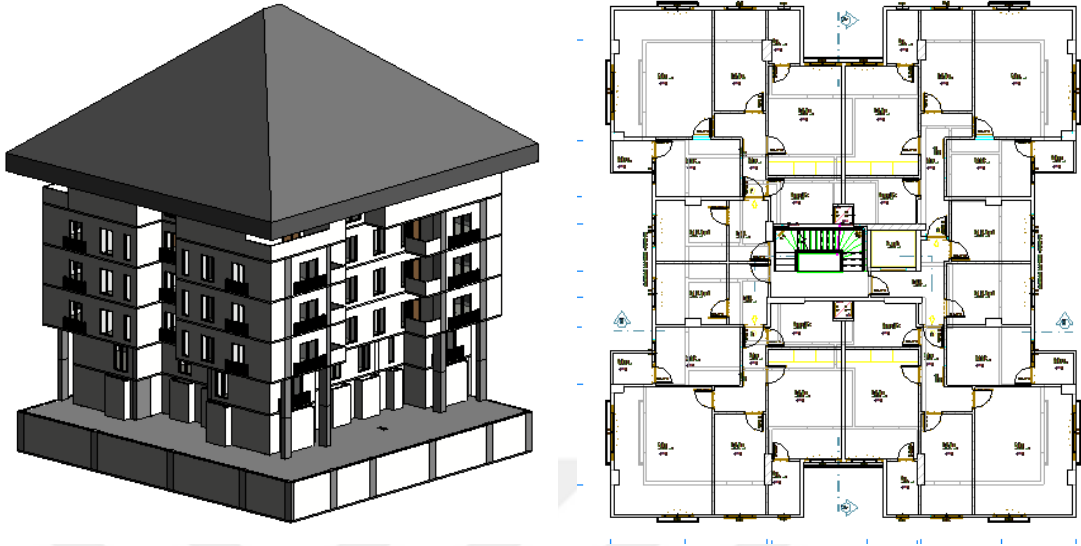
Figure 4.1 (a) 3D model of the case study building created in Autodesk Revit 2018, and (b) identical floor plan
