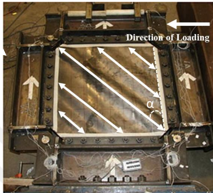
Figure 1.4. Tension field mechanism (Webster, 2013)
