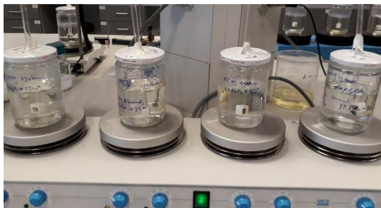
Figure 2-2 Experimental set up for static corrosion testing
