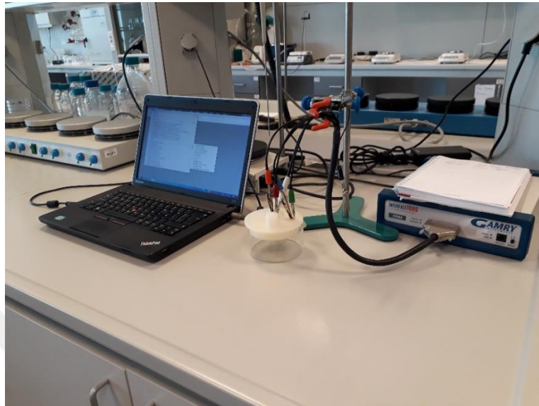
Figure 2-1 Experimental set up for electrochemical corrosion testing
