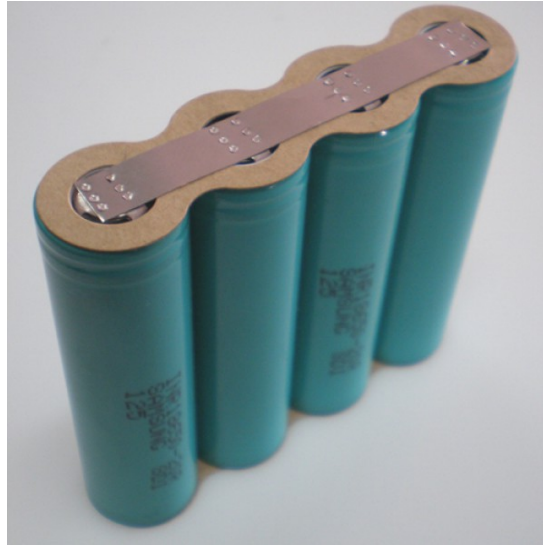
Figure 3: Connected Cells via Spot Welding
