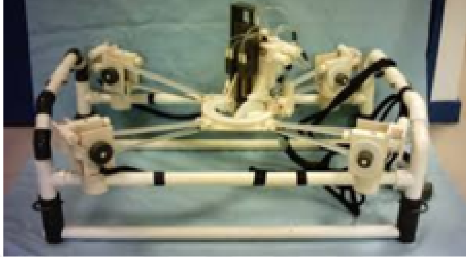
Figure 9: Light Puncture Robot as an example of patient attached surgery robot. [9]
