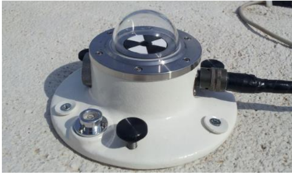
Şekil 3.20. 8-48 Model Black And White Pyranometer (The Diffuse Pyranometer)
