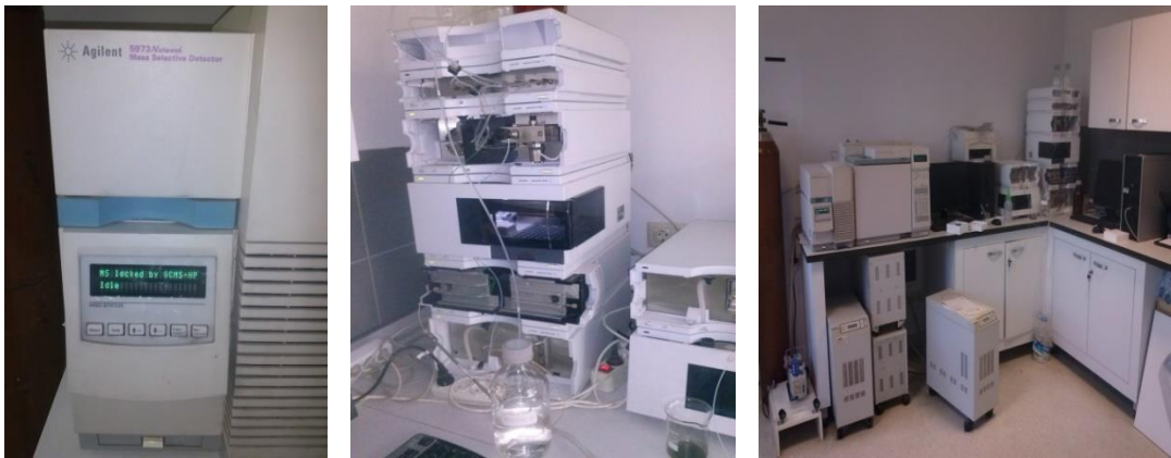
Fotoğraf 4.6. Agilent 6890N Network Gas Chromatograph ve Agilent 5973N Network CI/EI Mass Selective Detector
